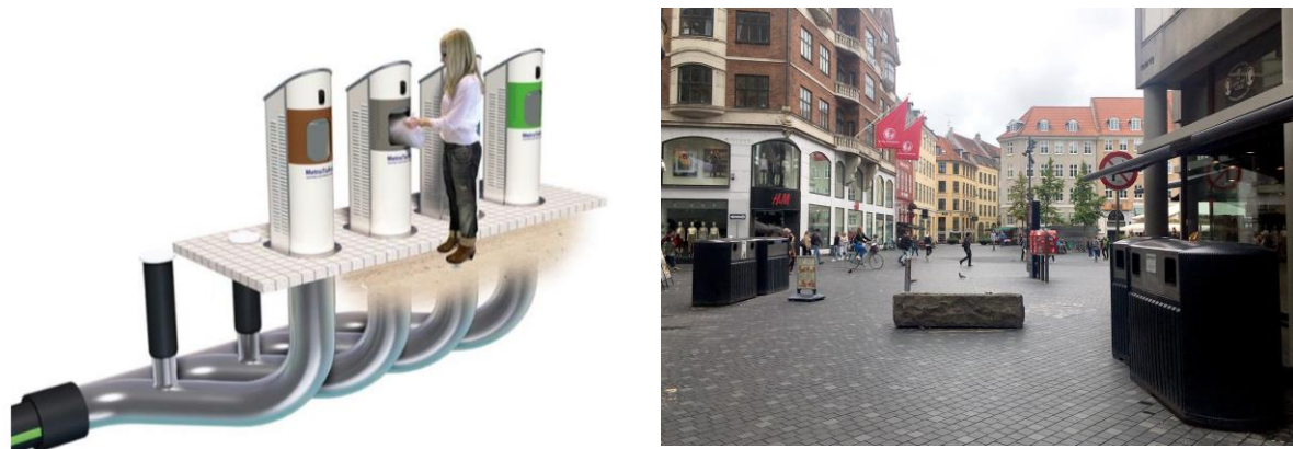
Figure 13. Public collection point (a) with suction system in Helsingør (for medieval towns with constricted space and pathways) 6 and (b) public collection points in Kulturvet, central Copenhagen 7
